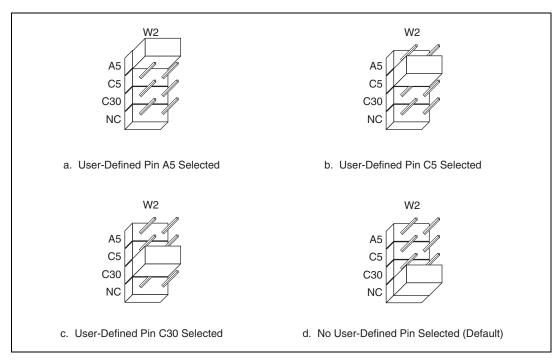
Figure 4-3. VME-MXI-2 Intermodule Signaling Settings
